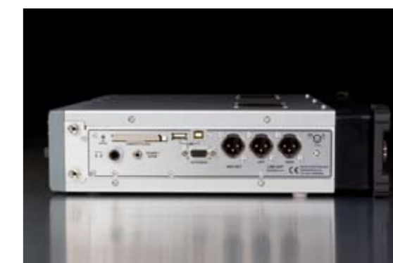
On the left and right sides of the machine: Inputs, DC supply and time code connectors, outputs, compact flash slot and communication ports
